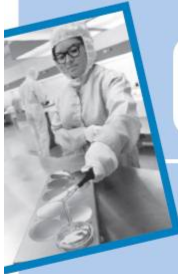
1976 An operator in an early bunnysuit shows how a 4-inch wafer is prepared for a positive acid spin.
